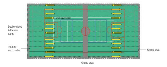
We recommend a dual—component epoxy glue, GreenLay Glue, reference Component A 1551057 Component B 1551058 — quantity to be applied, with a thin set of teeth spatula, between 300 and 350 gr per sqm. For a good installation you must carefully follow the manufacturer recommendations in particular, the waiting time before applying the covering. Then the surface with a roller to eliminate any bubbles that might remain between the sub—floor and the covering.
