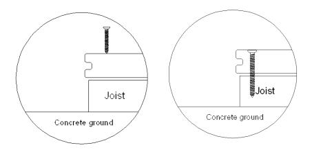
After the first deck is fixed, the rest decks to be fixed by screws and clips in turn
