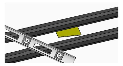
Attention: it is required that the deck surface is mounted flat and no water can collect on the surface or in the chambers. If water collects in the chambers for a long period, the board may start bending and waving because of the moisture expansion.
