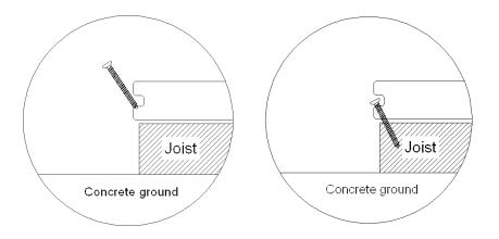
3C. Without starting clips, but screw from the top First, from the top of the deck, predrill a hole for the screw and into the joist; Second, fix the screw into the hole(see below pictures).
