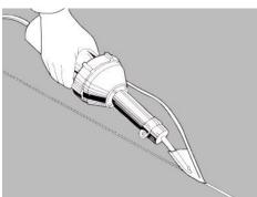
Weld with hot—air and Tarkett Speed Welding Nozzle. Carry out a test welding on a left over piece before commencing work, to adjust speed and temperature **Important:**When welding iQ Megalit, a Tarkett Speed Welding Nozzle or equivalent should be used.
