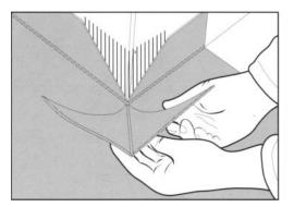
The triangle can now be folded and placed on the corner. It will overlap the coved floor. Cut through the overlapping material to make a tight fit.
