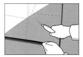
When fitting an out–corner, the sheet is folded against the corner and cut about 5 mm( $\frac{1}{4}$  in.) from the floor. The guidelines in the picture show the corner on the sheet and the position of the cut at about a 45–degree angle. Then a diagonal cut is made as shown.
