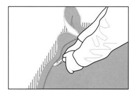
Avoid sharp creasing tools. When coving we highly recommend to use a Tarkett Hockey Stick or a Tarkett Corner Roller to press the material firmly into the juncture between the floor and wall. In areas where one sheet is sufficient to cover the subfloor, the adhesive can be applied over the entire surface area before installing the sheet. Although this requires experience, it is the fastest installation method.
