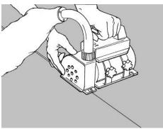
The sheets are hot welded. Do not weld until the adhesive has bonded completely, wait 24–48h. The joints are chamfered or grooved to about ¾ of the thickness using a hand grooving tool or machine prior to welding.
