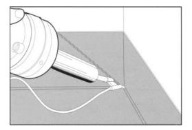
Use a hot–air gun for welding with thread at in–corners and out–corners. Tarkett Speed Welding Nozzle is specially designed for welding vinyl floors. For a perfect job, the Tarkett Swan Neck is required to effectively seal all seams nearest to the floor.
