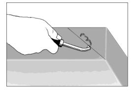
All seams on floor and coving must be grooved before welding.
