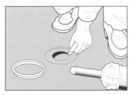
Around flush drain openings, heat the sheet and mark the location of the drain using a clamp ring. Then cut a small hole in the centre of the drain within the mark. Heat the flooring and press the clamp ring down into the edge of the drain. When using an adjustable clamp ring, make sure it fits tightly. Trim the material around the perimeter of the ring.Alternatively; use cutting tool as per recommendation from the drain manufacturer.
