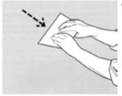
Press the sheet firmly using a piece of board with rounded edge or equivalent tool. Work from top down and from the middle to the sides of the sheet.
