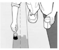
Apply adhesive to remaining area of wall and position sheet. Heat and stretch slightly the wall material around the corner at the same time as it is pressed firmly into the adhesive.
