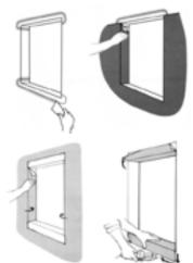
For best result , extra heating and pressing is necessary to secure a good bonding at overlapping areas.
