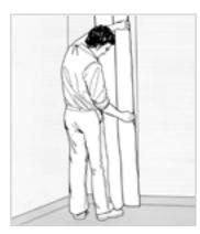
Back roll the wall material (face in) in the long direction. Place edge of wall material on plumb line and unroll into adhesive. Roll out the sheet little by little into the adhesive.
