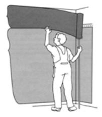
Be extra careful when washing off residues of adhesive at the border's overlap. Use clean water and a detergent suitable for removing adhesive
