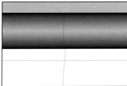
While the adhesive becomes tacky, the sheets are cut. The sheets should be cut longer than the room length to allow sufficient material for coving. When a sheet fits the width of the room, mark a cross mark on the bottom of the material and the subfloor to indicate the center. This will help you to place the sheet in its exact position. The cross marks are to coincide at installation.
