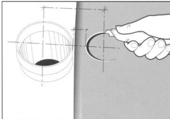
Around drain pipes, fold the sheet against the pipe and mark a line on the material where the center of the pipe is. Cut a hole about 25 mm (about 1 in.) smaller than the diameter of the pipe. As shown, cut the hole at the start of the fold. Heat the sheet vinyl and press it over the pipe. trim off excess material with a hook knife so that the break in the pipe wall is cleared.
