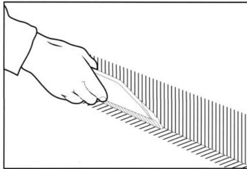
Using a straight edge and pencil, mark at a height of about 10 cm (approx. 4 in.) all walls where the flooring will be coved. Apply the adhesive on the walls up to the marked line, using a finenotched trowel. Spread some of the adhesive out onto the floor, as shown in the picture.
